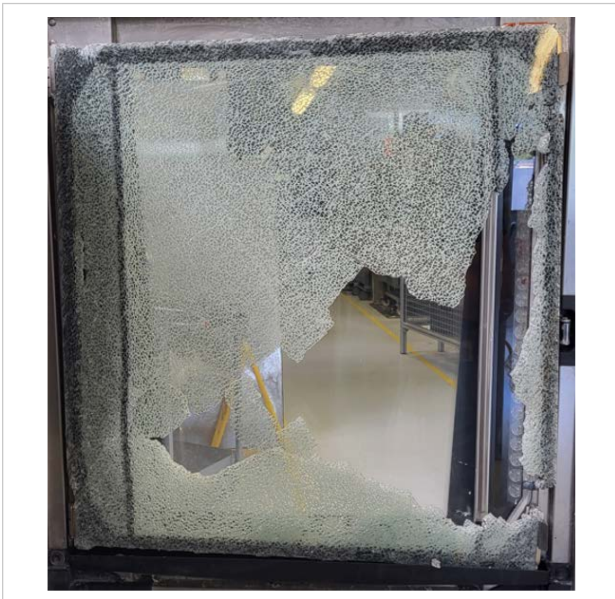
Pict. 2: Glass breakage on the inside
