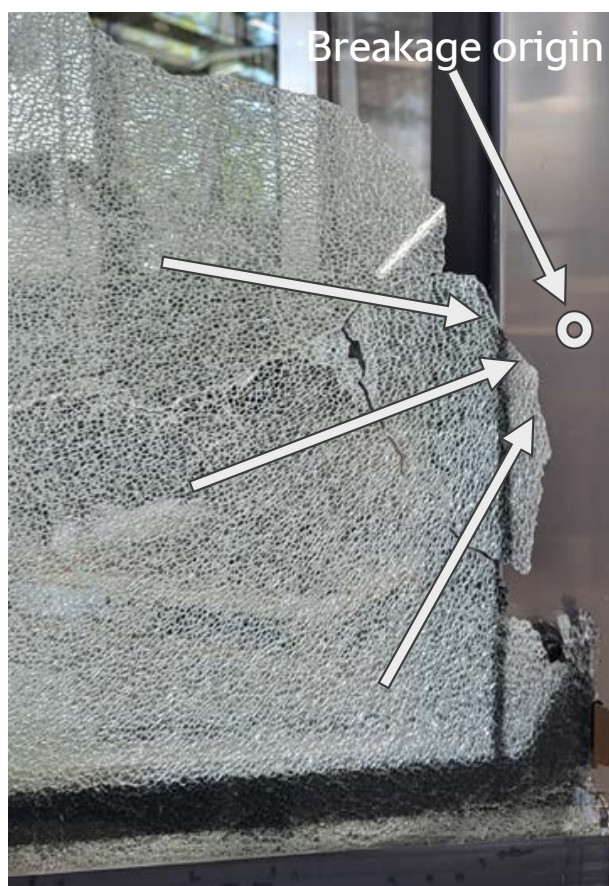
Pict. 6: Possible origin of breakage
