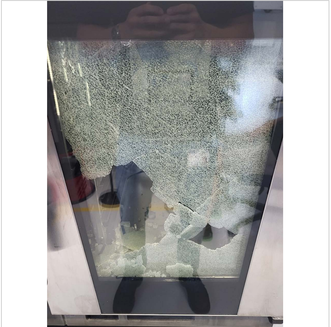
Pict. 1: Documentation of glass breakage from the outside
