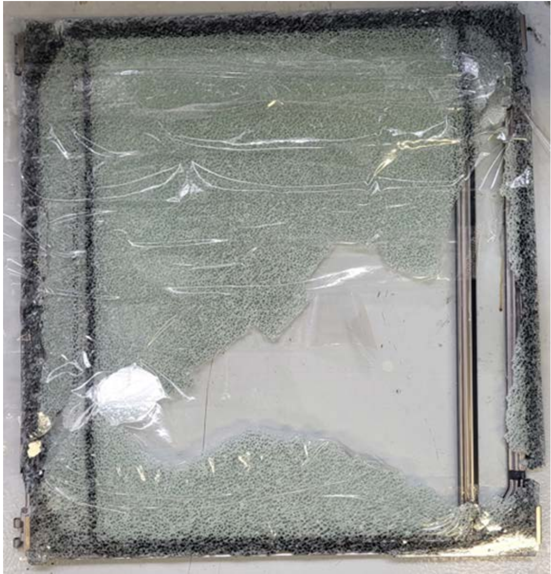
Pict. 3: Inner pane secured with adhesive tape when removed
