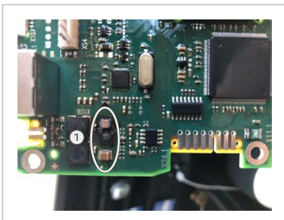
1 Faulty component on the PCB
